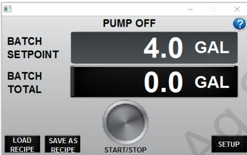
The BATCH SETPOINT and BATCH TOTAL are shown on the RUN Screen.
