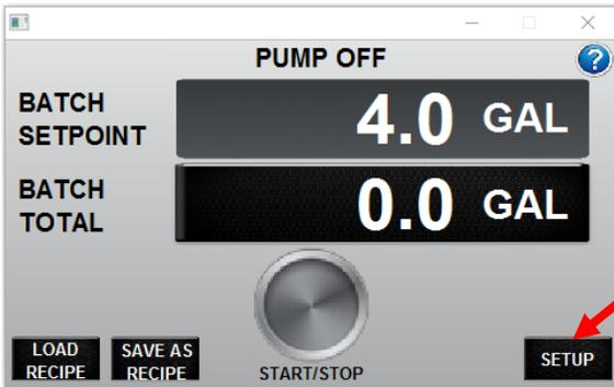
To navigate to the operational settings screen, press the SETUP button on the RUN screen.
