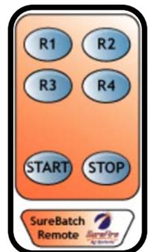
The START and STOP buttons on the remote control will always start and stop the current batch even if R1, R2, R3 and R4 are DISABLED.
