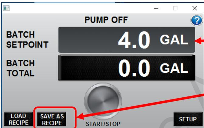
To SAVE RECIPE first set the Batch Setpoint setting. Here the batch size is 4.0 GAL. Then push SAVE AS RECIPE.
