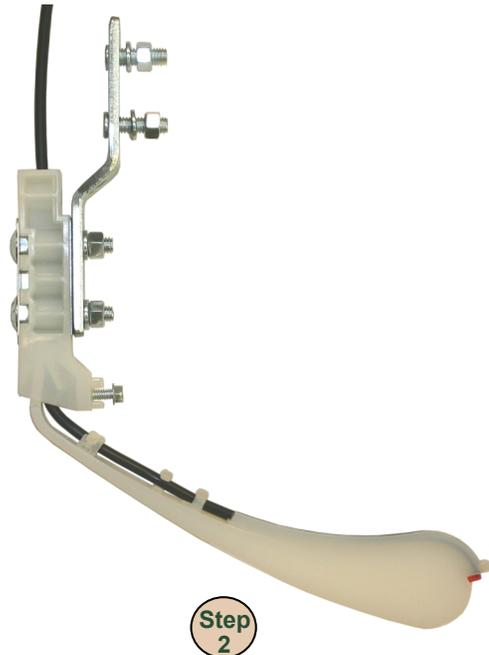
Bolt the Tube Guard and the Steel Bracket to the firmer using the 2-  $\frac{3}{8}$  x 2" carriage bolts and 2 lock washers provided. The Tube Guard is always placed on the tube side of the firmer.
