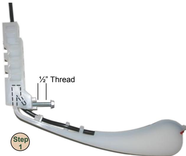
Assemble 2-piece liquid firmer by inserting the Tail into the poly base as shown. Make sure tension screw is below the tab on Tail section.
