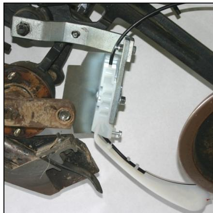
After mounting the first unit on the drill, measure the height from the Firmer's tension screw to the ground. That distance should be approximately 4" to 4-1/2". Repeat the procedures for each unit.
